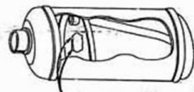
Insert a steel cable (diam. 7mm) into the tail pipe.
